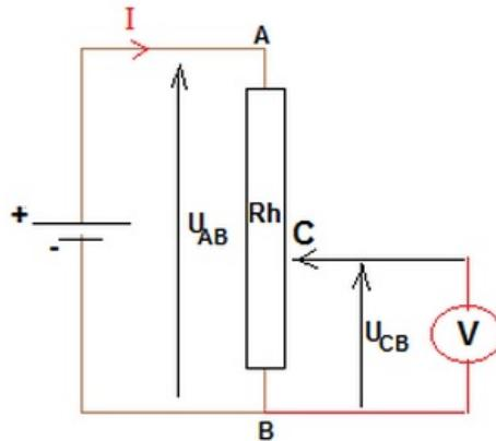
$$U_{CB} = R_{CB} \cdot I = R_{CB} \cdot \frac{U_{AB}}{R_{AB}} = U_{AB} \cdot \frac{R_{CB}}{R_{AB}}$$
