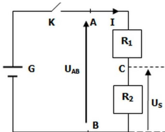
$$U_s = R_2 \cdot I = R_2 \cdot \frac{U_{AB}}{R_1 + R_2} = U_{AB} \cdot \frac{R_2}{R_1 + R_2}$$
