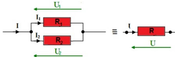
$$\begin{aligned} I &= I_1 + I_2 \\ \frac{U}{R} &= \frac{U}{R_1} + \frac{U}{R_2} \\ \frac{1}{R} &= \frac{1}{R_1} + \frac{1}{R_2} \end{aligned}$$
