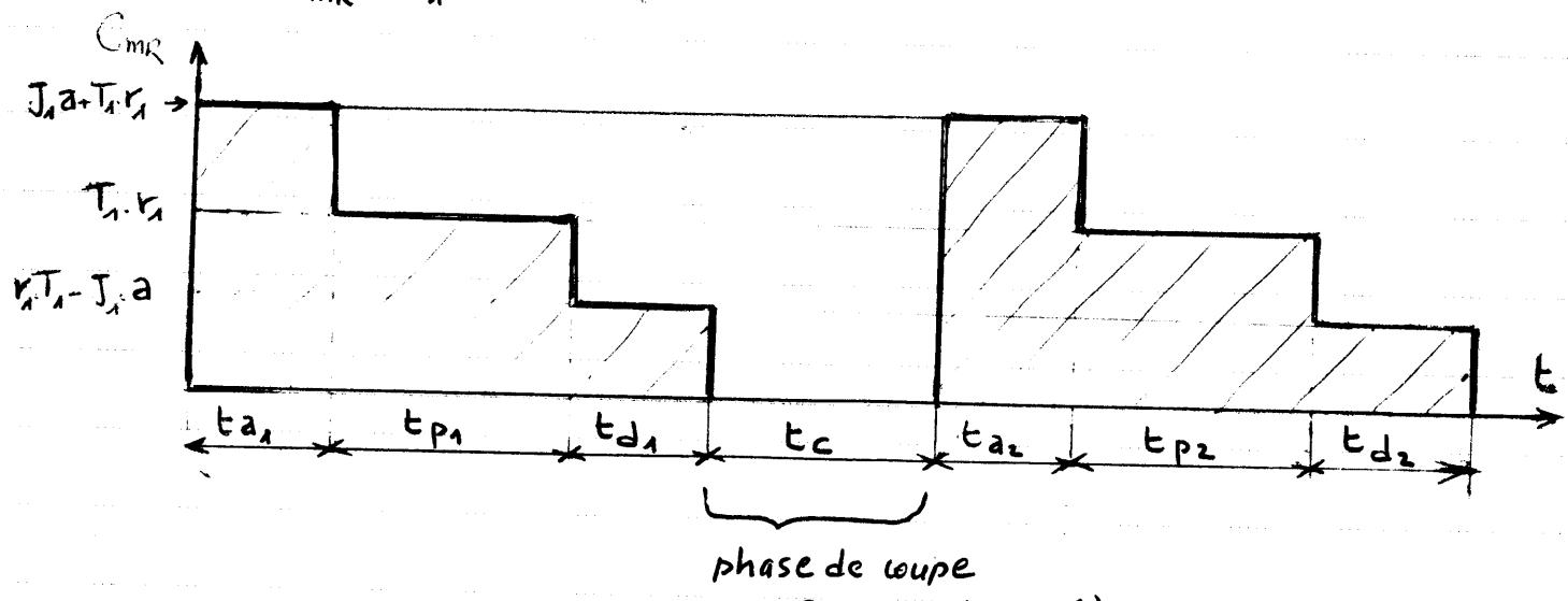
\*  $P_m^{\max} = C_{MR}^{\max} \cdot \omega_{\max} = (J_1 \cdot \alpha + T_1 \cdot r_1) \cdot \omega_{\max}$
