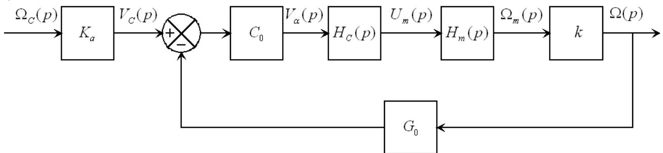
$$FTBF(p) = \frac{\Omega_m(p)}{\Omega_c(p)} = \frac{\Omega_m(p)}{V_c(p)} \times \frac{V_c(p)}{\Omega_c(p)} = \frac{C_0 H_c(p) H_m(p) k}{1 + C_0 H_c(p) H_m(p) k G_0} K_a = \frac{C_0 k K_a H_c(p) H_m(p)}{1 + C_0 G_0 k H_c(p) H_m(p)}.$$
