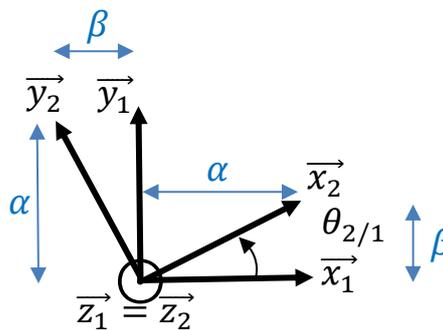
$$\begin{aligned} \vec{x}_2 &= \alpha \vec{x}_1 + \beta \vec{y}_1 \\ \vec{y}_2 &= -\beta \vec{x}_1 + \alpha \vec{y}_1 \end{aligned}$$
