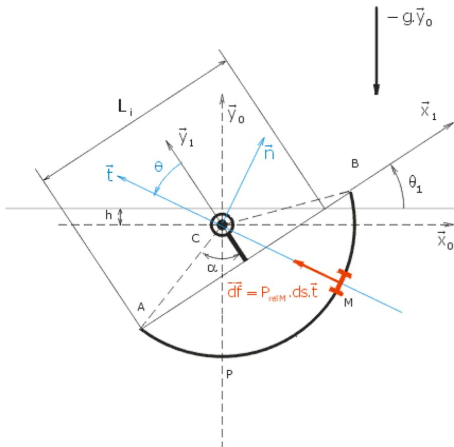
$$M \left\{ dT_{Eau \rightarrow Cylindre} \right\} = \begin{Bmatrix} -P_{rel M} dS \vec{t} \\ \vec{0} \end{Bmatrix}$$
