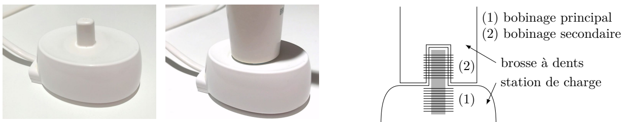
Figure 9 Station de charge
