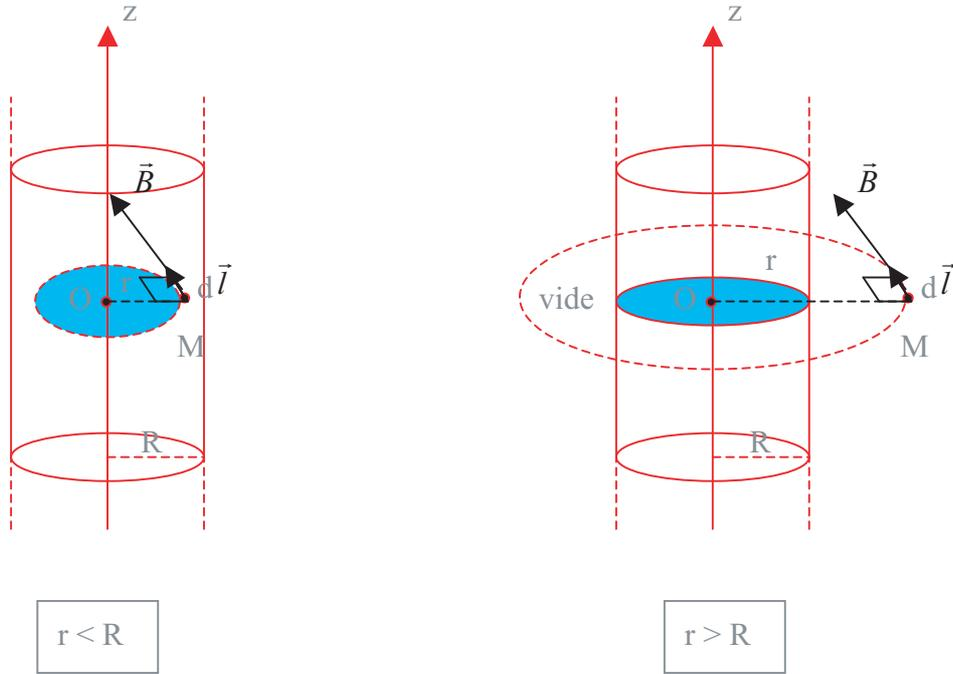
$$2.2 \quad d\vec{F}_m = \vec{j}d\tau \times \vec{B}_{int} = \frac{I}{\pi R^2} \vec{z}d\tau \times \frac{\mu_0 I}{2\pi R^2} r \vec{e}_\theta = -\frac{\mu_0 I^2 r}{2\pi^2 R^4} d\tau \vec{e}_r$$
